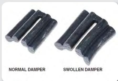
For this reason it's always important to follow the manufacturer's recommendation for lubricants. For example, with Yamaha's Talon propeller with SDS, it's important to use only Yamaha WR No. 2 grease to avoid possible damage to the dampers. Be sure to check the appropriate Owner's Manual if you have any questions.
