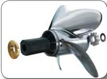
For propellers with universal hubs you will need to look for any signs of cracking or splitting in the hub. These hubs are usually made of a hard plastic or Nylon type material molded around a brass spline. To limit any excess wear on the hub, do not remove it unless you see signs of damage.
