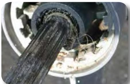
With the propeller off look over the propeller shaft and gearcase seals. If any fishing line or debris is wrapped around the shaft or even stuck in the seals, this would be a good time to contact your local Yamaha dealer to have the gearcase pressure tested. If no debris was found then you should proceed with cleaning the old grease from the shaft. Use a light solvent and a rag to wipe down any old grease.
