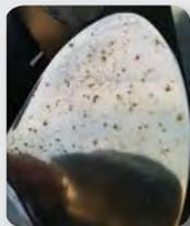
First off, remember that propellers are "stain-less," not stain-proof. There is a measure of iron contained in any stainless steel propeller in order to maintain the necessary hardness in metallurgy. Therefore, depending on how you use and care for your propeller, surface discoloration can appear over time. It doesn't affect performance, just appearance.
