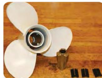
brass-splined hub and remove the dampers. Wipe the inside of the hub clean and prepare the new dampers. Using Yamaha WR No. 2 grease, apply a liberal coating to the new dampers. Place one damper over each outer spline on the brass hub (There are 3 outer splines). Gently push the hub and dampers into the propeller using the aft spacer to fully seat the hub. Now just grease the propshaft and you are ready to reinstall your Talon propeller.
