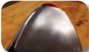
The other location where cup can be placed is at the blade tip, as shown in the adjacent image. Cupping in this area essentially adds rake to the propeller. Cupping at the blade tip will have a large effect on how the propeller grips the water and provides lift for maximum hull efficiency.
