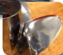
There are many parts of a propeller that affect the way it performs, but one that is commonly misunderstood is the cup. Most often cup is confused for the dished out portion of the blade's face, or pressure side. In fact, the cup is found along the trailing edge of the blade and the blade tip. Cup is commonly modified by propeller repair shops, but how do these changes affect the propeller's performance?
