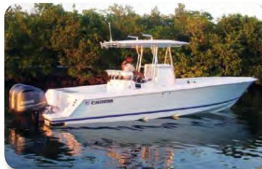
Due to their speed and responsiveness, stepped hulls sometimes exhibit characteristics that give the captain the impression that the boat is unstable or too touchy at the helm. To help combat this feeling, four-blade propellers such as the Yamaha Saltwater Series HS4 (V6s), XL4-HP (V8s), and the Turbo Fusion 4 are often used. The four-blade propellers provide the added grip and stability that stepped hulls sometimes need.
