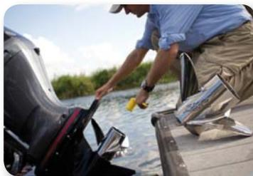
First, make sure your boat's hull is clean and structurally sound and that the engine(s) runs correctly. Then, in your normal boating environment, run your boat wide-open with your average load and in average conditions, trimmed for
