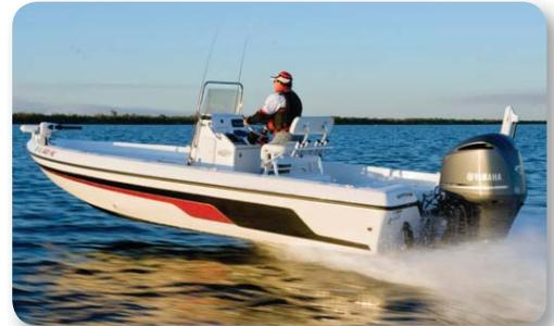
One particular outboard/propeller combination we've found that works well on these larger bay boats is Yamaha's big bore 4.2L V6 Offshore four stroke outboard mated to a Turbo Offshore I propeller. The large diameter, four-blade design of the Offshore I creates both stern and bow lift. This allows it to move large loads quickly, and keep the boat on plane at slower engine speeds, making it both effective and economical. It can also help minimize the draft of the boat while on plane.
