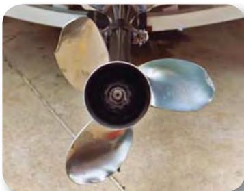
**2 Impacts.** Obviously, any form of impact is going to be detrimental to your propeller's performance. Even small knicks or dings in a blade can lead to poor performance and even catastrophic cavitation. If you have impacted something to the point that you have bent or broken a blade or blade tip, you'll realize poor performance coupled with potentially damaging vibration. This condition can lead to expensive prop shaft, bearing, or gear damage, and that's time you're off the water.
