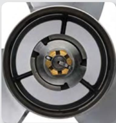
Make it a habit to grease the prop shaft with a high-quality marine grease while you have the prop off, and *replace* the cotter pin instead of reusing it. That \$1.50 you saved by reusing the pin instead of replacing it won't come close to getting you home if that old pin breaks, and it very well might allow your nice, shiny prop to slip off into the depths!
