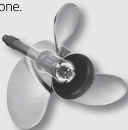
Propellers equipped with this system use a unique, splined rubber hub and special aft spacer on the propeller shaft to distribute and absorb the forces and the resulting sounds and vibration, which are normally associated with shifting an outboard into gear. The result: far quieter and smoother clunk-free shifting.
