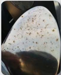
First, it's important to remember the propellers are stainless not stain-proof. We test and re-test our props to help ensure maximum resistance to corrosion while still maintaining the necessary hardness in metallurgy. But because there is a measure of iron contained in any stainless steel propeller, surface discoloration can appear over time. This surface discoloration is somewhat normal in certain instances. It doesn't affect performance, just appearance.
