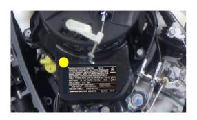
**NOTE:** Modified units still in their crate can be identified by blue seal marks on the labels as shown below:
