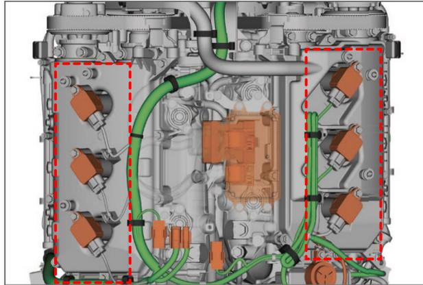
4. Install the ignition coil cover and flywheel cover. Mark the ignition coil cover with a white paint pen as shown in the *Identification Procedure* on page 18.
